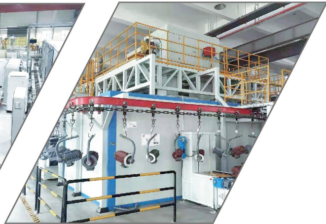
悬挂链电机喷漆线
