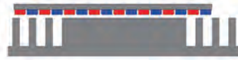
图 4 直线电机动子在段间切换时齿槽效应模型 Fig. 4 Model of the cogging effect during segments switching of linear motor
