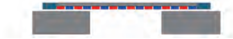
图 11 添加辅助结构的直线电机段间切换时边端效应模型 Fig. 11 Model of end effect during segments switching of linear motor with adding auxiliary structure
