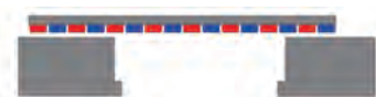
图 5 直线电机动子段间切换时边端效应模型 Fig. 5 Model of end effect during segments switching of linear motor
