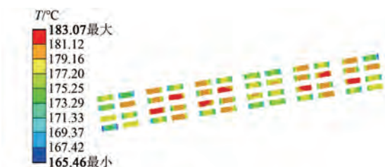
图 10 满载永磁体温度分布 Fig. 10 Temperature distribution of the permanent magnet at full load
