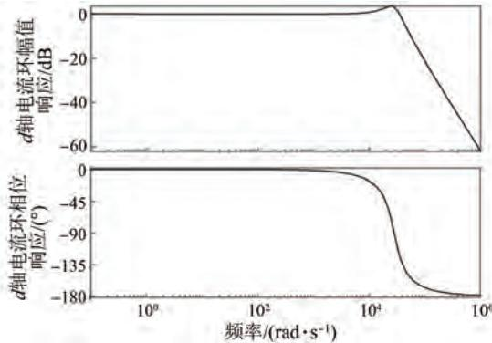
图 11  $d$  轴电流环传递函数伯德图Fig. 11 Bode plots of transfer function for  $d$ -axis current loop
