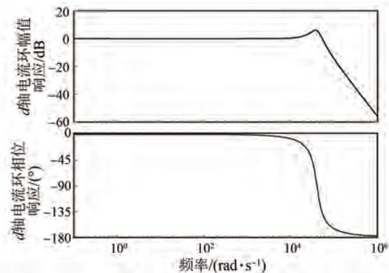
图 12  $q$  轴电流环传递函数伯德图Fig. 12 Bode plots of transfer function for  $q$ -axis current loop
