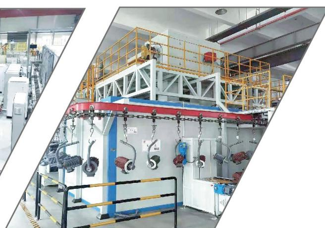
悬挂链电机喷漆线
