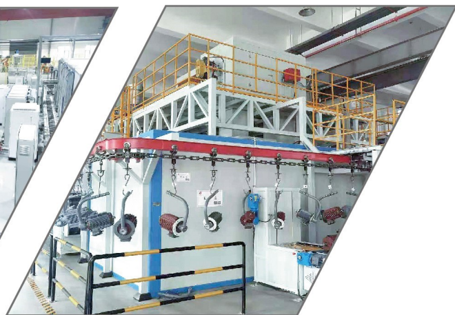
悬挂链电机喷漆线
