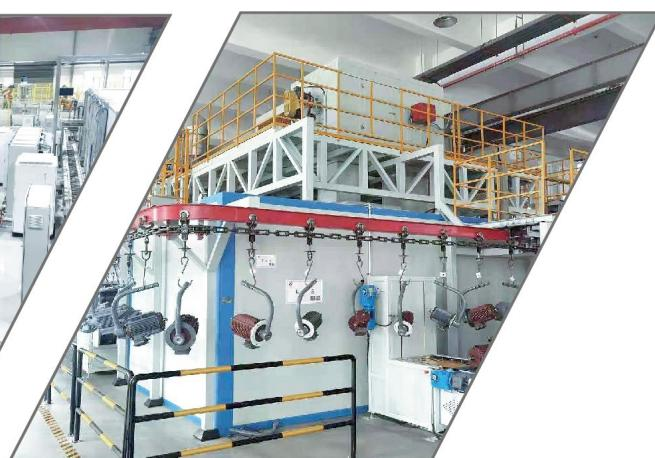
悬挂链电机喷漆线
