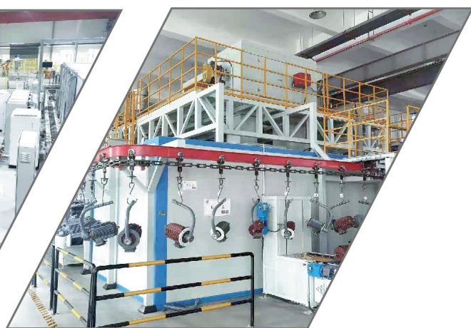
悬挂链电机喷漆线
