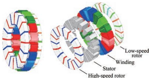
**Fig. 1 Three-dimensional model of a poly-magnetic axial magnetic gear composite motor**
